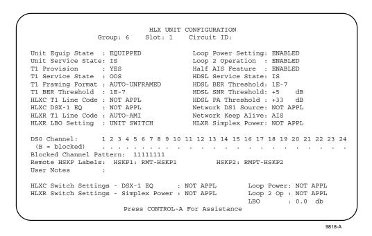
Figure 531-2. HLXC Unit Configuration Screen
